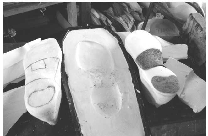
51 There are two ways to proceed. First, is to make the shoe with the insert above so that the "mud" on the bottom has all of the appliances shapes. Or secondly, to make the shoe the way as the old unaltered last without appliances.
