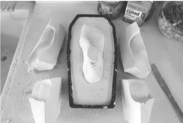
38 The top 4 negative cast pieces have been removed so you can see the new positive cast of a last.
