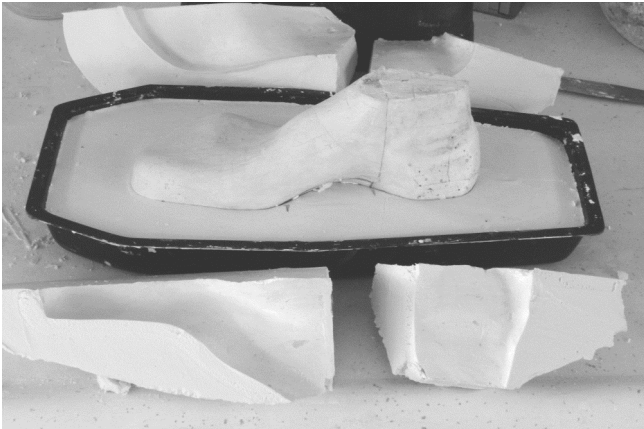
32 After the top plaster has firmed sufficiently, it is removed. Now we have 5 pieces of the negative cast and 1 piece of the positive cast, which is also a last.
