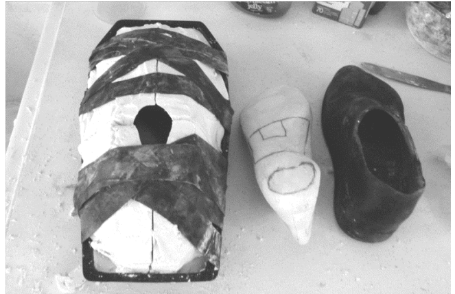
35 The 5 pieces of the negative cast have been put together; they are on the left. The unaltered last is in the middle. The old shoe from which the appliances came, is on the right.
