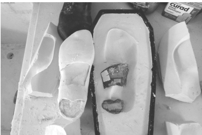
40 The appliances have been removed from the positive cast of a last.
