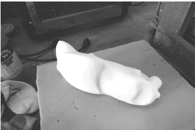
50 The Pe-Lite® has taken the shape of the last without the appliances.
