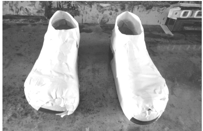
8 We need to carefully use painters masking tape to seal up these shoes and build an extension on top. We are very careful to not distort the shoe while masking.
