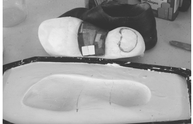
33 Now, we are going to make a new positive cast, which will also be a last with two added parts or appliances as prescribed by the Doctor. They are the arch support and a heel block.
