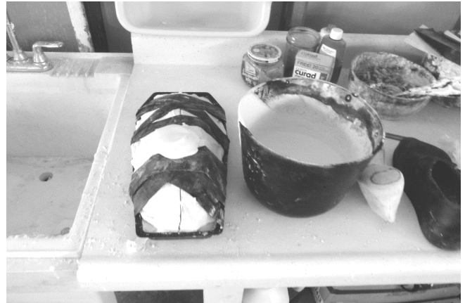
37 The plaster has been poured into the 5-piece negative cast.
