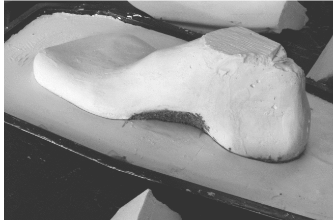
43 I have just pushed the wet "mudded" last into the bottom negative cast.
