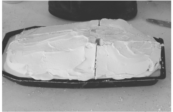
31 The top of last is covered with wet plaster and as it firms it is quartered with a butter knife.
